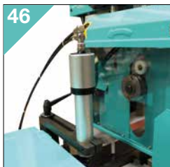
691100 - SIRIO Morsa verticale pneumatica. Vertical pneumatic vice.
